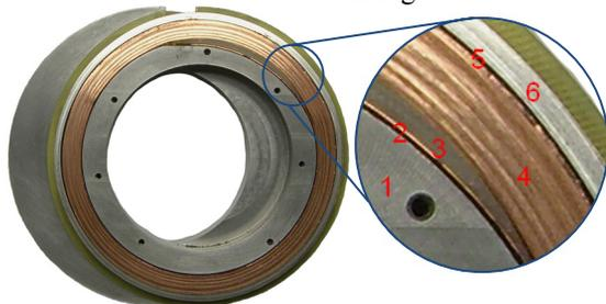
Figure 6: Double-pancake technological model: 1) inner support ring; 2) coil inner ground insulation; 3) spacer for the first turn; 4) coil; 5) coil outer ground insulation; 5) stainless steel bandage outer support.
