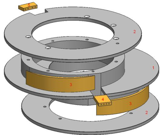
Figure 3: Expanded view of a double pancake unit: 1) inner support rings with flange; 2) side flanges; 3) spacer for the first turn and splice accommodation; 4) insert with holes for the inner splice cooling and support; 5) inserts for the outer splice support.
