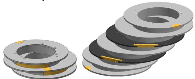
Figure 4: The double pancake unit (left) and three double-pancakes connected together (right). The dark grey flanges accommodate the splices between units.
