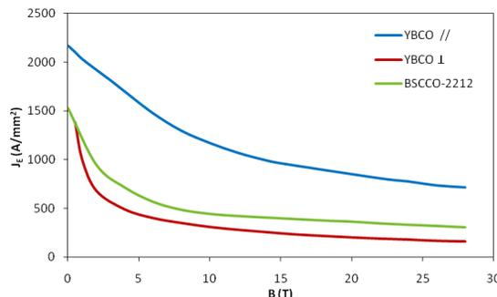
Figure 1:  $J_E$  vs.  $B$  for BSCCO wire and YBCO tape.
