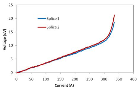
Figure 5: V-I curve at 77 K for each of the inner splices.
